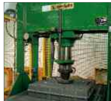
Tests su chiusura Load tests on access cover
